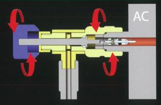
Internal pin activates refrigerant flow.
