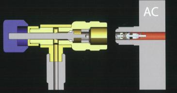
The fitting is screwed onto the service port.
