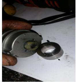
Step 5: Turn the ignition position locator. You should now feel spring tension from where the ON position is to the START/CRANK position is. Re-install to column, tighten m4x8 screw where roll pin 1 was and install UF-1. Refer to page 8 and 9. Finish.
