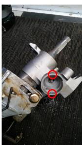
**Step 8**: Push the UF1 onto the steering housing.
