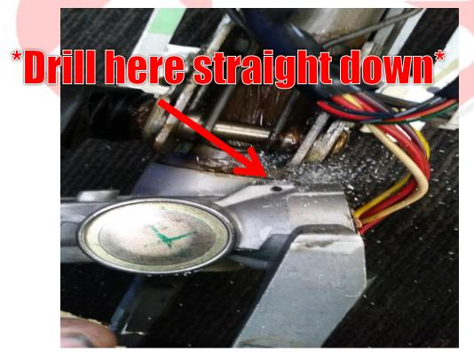
**Step 5**: Gently pry the electrical switch out as shown in picture if it hasn't already sprung out whilst drilling the hole.
