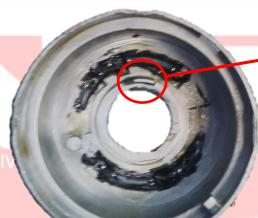
This very small diecast tab is the part which breaks or wears down inside the switch housing. If the vehicle is not returning from the start position this is the problem.
