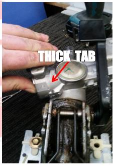
Step 9: Locate the 4mm hole in each tab and using a 4mm drill bit mark your holes only. DO NOT DRILL ALL THE WAY THROUGH. Ensure you apply pressure to the UF1 to ensure it is flush with the housing.
