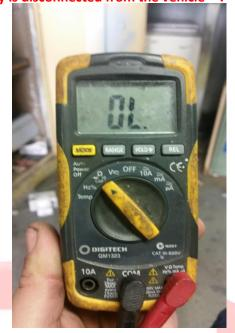
Step 2: .Probe Red wire with a green trace and white wire as shown below. Then turn key to ON position. You should here an audible beep. Turn to START and it should disappear and then come back when it returns to ON position. This is testing that the ON position is working when the key returns from START.
