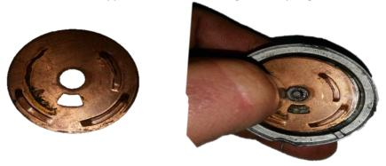
**Step 9:** Examine the wiring terminal insert, on 1x side there is a cut out which need to line up with locator on the switch housing. Line them up and proceed to push the insert into place.
