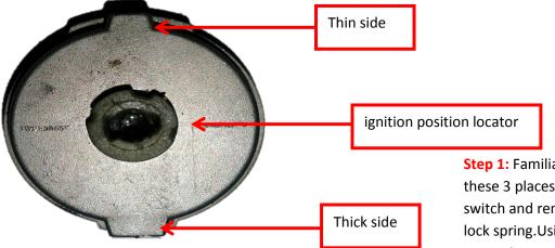
**Step 1:** Familiarise yourself with these 3 places on the ignition switch and remove the steering lock spring. Using a flat blade screw driver turn ignition position locator anti-clockwise until it stops.
