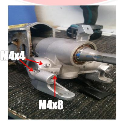
**Step 11:** If the electrical switch is in good working order it can now be fitted back into the column (it only goes in one way.
