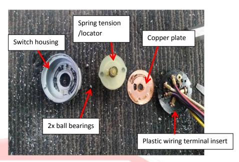
Step 2: Examine your switch housing if the spring return diecast tab is still present you need to Flatten with a punch in order to fit the FSR-1 insert.
