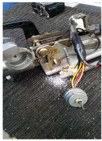
Step 6: Remove any debris and punch the remains of the roll pin out of the housing to ensure easier fitment of the switch later on in the procedure.
