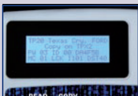
More detailed information on the original transponder, indicating the JMA transponder over the one to be cloned, and a guide of the steps to follow.
