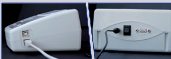
Only two cables: Power-Supply and Updating via USB.
