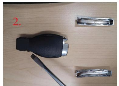
3. Remove bottom emergency blade housing using a small flat blade screwdriver or similar tool.
