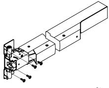
CHASSIS ASS'Y WITH 10# \* 3/4" FLAT HEAD SCREWS(4)
