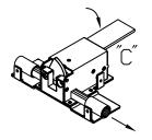
OPERATE LIFT ARM "C" TO ENSURE THE PROCESSING DIRECTION IS REVERSED.
