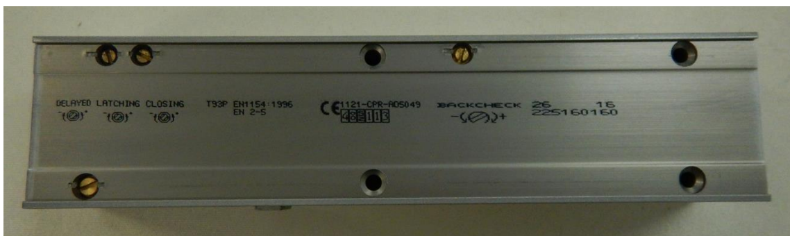
Figure 3 Uninstalled door closer
