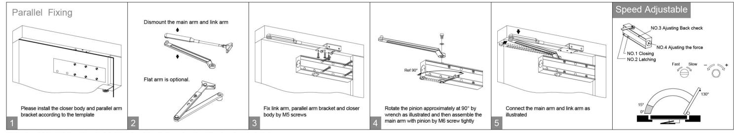
XIf the strength is too light, it could be adjusted at clockwise rotation. On the contrary, it could be done at counterclockwise.
