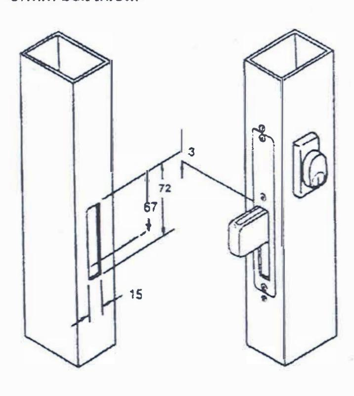
B. FOR SLIDING DOOR HOOK BOLT: Cut opening in door jamb to suit strike plate. Drill holes as shown. Fit strike assembly into door jamb and secure with screws. Attach strike cover plate.
