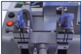
1 4-sided vices. Compatible with earlier duplicating machines such as Dakota, Titan, Saratoga...
