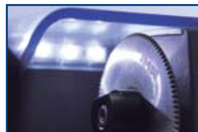
2 Low consumption LED lights to illuminate the cutting area. Ample protection from the milling cutter.
