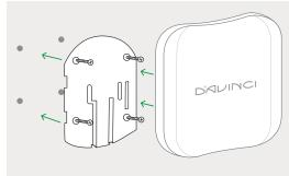
Fix the support to the wall using the supplied screws. Fix the Repeater on the support and tighten the locking screws.
