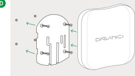
Fix the Lisa Panel Controll to the wall using the dowels and installation kit screws.
