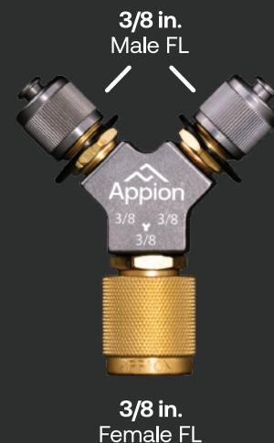
The Speed-Y™ comes in three different sizes, each featuring two male 3/8 in. flare fittings for service hoses. Available in 1/4 in., 3/8 in., and 1/2 in. female flare sizes, the Speed-Y™ can be used for various applications. Built with premium aircraft-grade aluminum, each Speed-Y™ is constructed to endure in the toughest of conditions.
