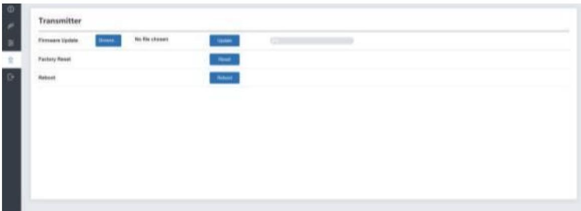
Click "Browse." to import the upgrade file and click "Update" to start upgrade. There will be a progress bar prompt during the upgrade process. When the progress bar reaches 100%, it indicates the upgrade is successful, and the device will be restarted automatically.
