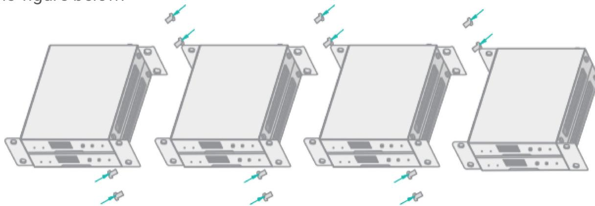
**Step 3:** Fasten screws between two 1U rack panels, so that eight products are mounted in a 1U rack, as shown in the figure below:
