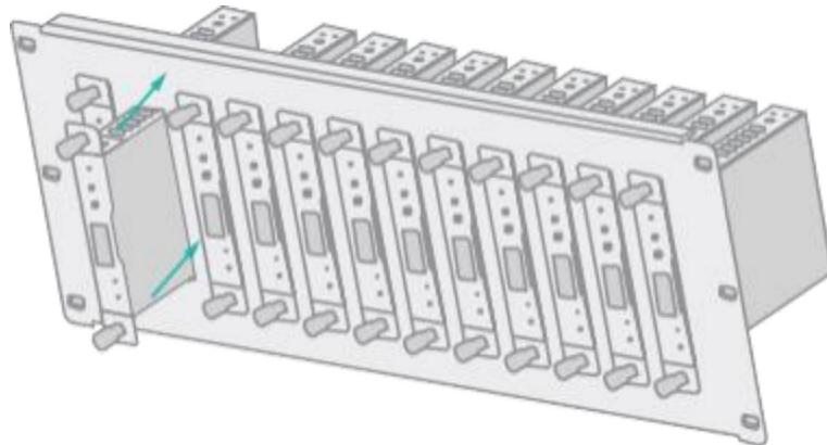
**Step 3:** Use screws to fix mounting ears on the rack to complete the mounting, as shown in the figure below:
