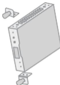
**Step 2:** Insert the product with mounting ears into a 4U rack (up to 12 units can be installed vertically), as shown in the figure below:
