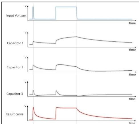
Much like the ‘adaptive attack’ feature, **Auto Release** is program dependant. This unique design utilizes a stack of three capacitors that are optimised for short, medium, and long, time constants. Their combination means that the faster the input transient, the faster the release time. The longer a signal remains above the threshold, the longer the resulting release time.
