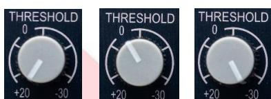
The maximum threshold of **-30dBu** is indicated at the 5 o'clock position.
