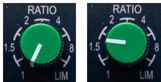
The **RATIO** pot determines the amount which the compressor will act upon (reduce) the signal above the Threshold. These two controls are used to form the overall gain reduction of the input signal.
