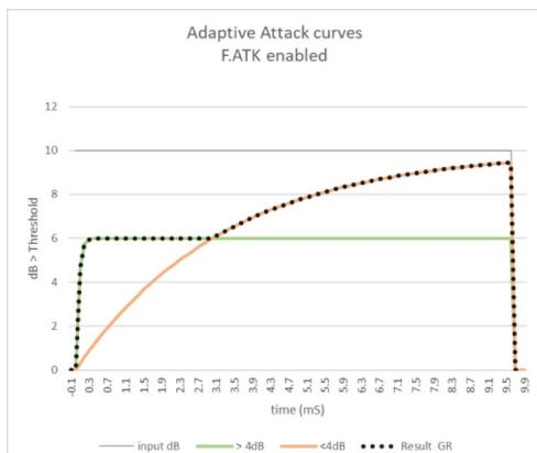
Once activated, **FAST** increases the range of combined adaptive attack time to provide an even faster response to the louder transients.
