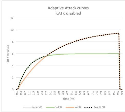
This adaptive attack mode allows louder transients to receive a faster attack time, and quieter transients to receive a slower attack time.
