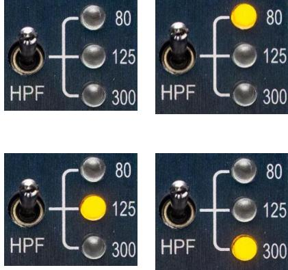
When HPF is engaged, a second order high pass filter is applied to the compressor sidechain, before VCA compression is applied. This feature can be used to prevent sonic material below the frequencies of **80**, **125**, and **300Hz** from triggering the compressor.
