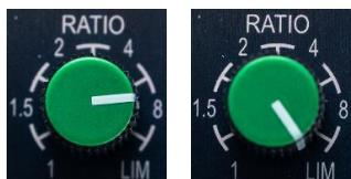
Turning the pot completely clockwise to 'Lim' (limiting) would mean that the audio above the threshold is completely reduced.
