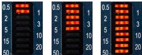
The gain reduction meter displays the total amount of **G/R** (Gain Reduction) applied to the signal due to the threshold and ratio settings.
