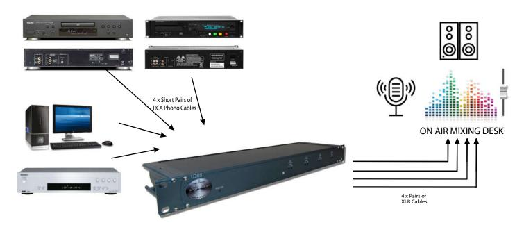
Many radio stations and studios incorporate mid level domestic audio equipment such as CD players & recorders, FM/ DAB Tuners, PCs tape machines etc as they provide reasonable value for money in comparison to professional versions. The output of such devices need to be correctly interfaced with a professional or broadcast audio desk.
