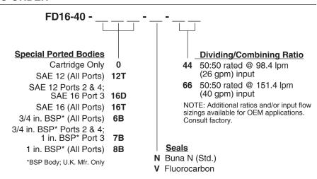
NOTE: Standard 16-size 4-way bodies should not be used for flow dividers. See special flow divider bodies, page 8.016.1.
