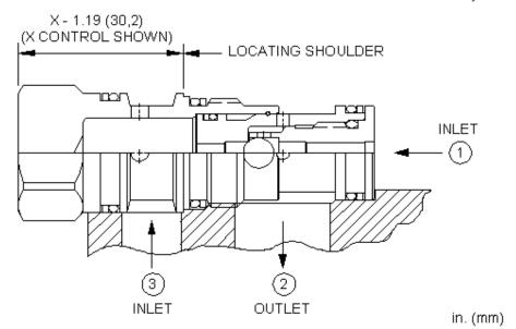
The single ball shuttle connects the higher of two work ports to the signal or common port. The signal is sensed at port 2.
