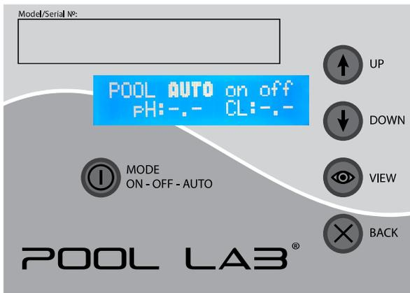
When an ASP is connected to the Pool Lab chlorinator the bottom line of the display will show the pH and Chlorine levels. The values will initially be “-.-” indicating that the value is unknown until the first water test occurs.
