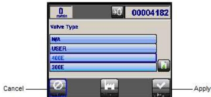
**i** If the default valve type that appears is "not applicable" (N/A), use the Plus/Minus buttons to scroll through the list of valve types available.
