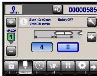
3. Press the Right Arrow Button until the scroll right button is highlighted, and then press Okay to view the Delay Length for pattern 2. The control automatically fills in the Delay Length for pattern 2 (so the next pattern does not interfere with the previous pattern). This number can be adjusted if desired.
