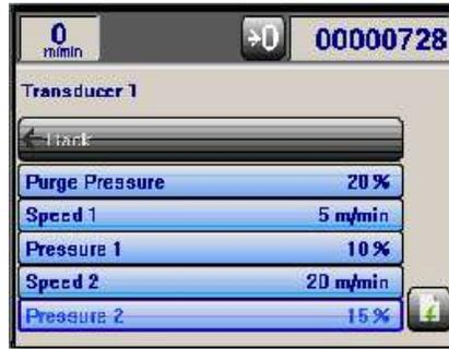
**Purge Pressure** - The pressure setting when the machine is at zero speed.
