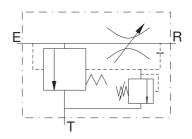
**DESCRIPTION:** The FCV34-3R valve is a 3 port by-pass style flow control for use in high pressure hydraulic circuits. It features flow rate to 150 litres/min., tamper resistant pressure relief adjustment, and a stainless steel adjusting mechanism.
