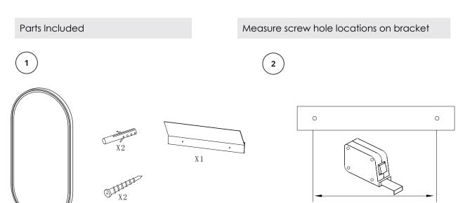
When marking for screw, ensure level with mirror rear bracket
