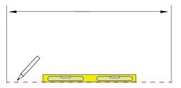
Drill holes for mounting screws provided, ensure these are drilled into supporting wall (throughmasonary, brick wall or noggins to support the cabinet load).
