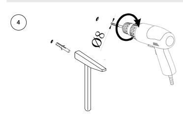
Drill the screw into the wall
