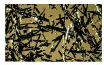
Cavex Avalloy. Lathe-cut, gamma-2-free. The economical choice thanks to the low silver and high copper content. A packable amalgam (with a feel like "crumbling snow") with no risk of discoloration.
