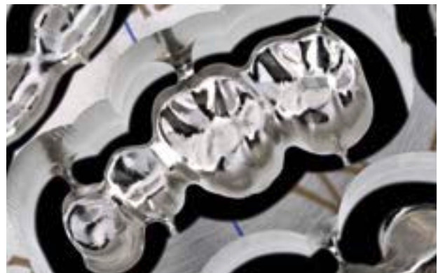
Very smooth and shiny surface (CoCr milled).
