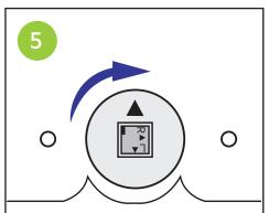
Manually move the top plate to match the inside square, this so the arrow faces upwards.
