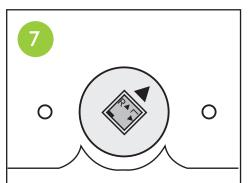
Pull the spindle only halfway out and rotate the top plate only clockwise, until it can go no further. Your mechanism should look like the image above.
