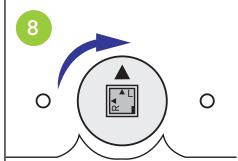
Push the spindle all the way in again and rotate both plates clockwise until you see the arrow at the top like the image above.
