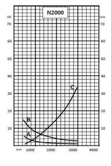
(i) To assess maximum distributed beam load at allowable stress, determine from Graph "A" (ii) For maximum axial load, determine from Graph "B"
