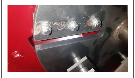
Using a 13mm spanner, loosen the nut that connects the chipper blade to the flywheel.
