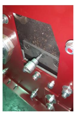
In order to fully remove the nut and bolt, use a 6mm Allen key to counter the force from the spanner. Remove the nuts and bolts from the chipper blade. Once all three have been removed, take out the chipper blade. The chipper blade will come out of the chipper chute entrance. When putting the blades back in you should always replace the nuts and bolts and Loctite the thread for safety.
