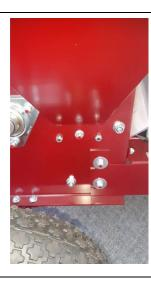
Remove the chipper chute using a 13mm spanner to give access to the bolt holding the chipper blade.
