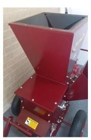
Take off the hopper plate of the machine using a 13mm spanner. Place a bar through the flywheel. Ensure that the flywheel doesn't rotate when this bar is in place by pulling the engine cord.
