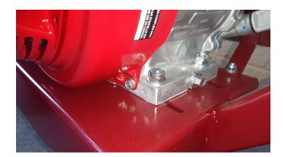
Using a 17mm spanner, loosen the nuts that connect the engine to the frame of the machine.
