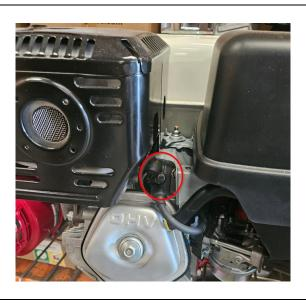
Disconnect the spark plug to ensure that the machine will not receive power whilst you are working on the flywheel
