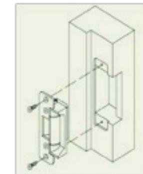
Mounting installation on wooden door frame
