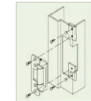
Mounting installation on metal, aluminum or PVC door frames
