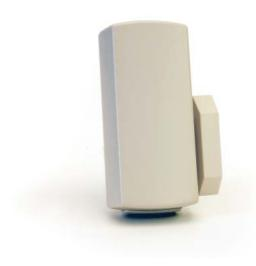
The Inovonics door/window transmitter with reed switch includes a built-in, side mounted magnetic reed switch, with a magnet that supports a 5/8" gap.
