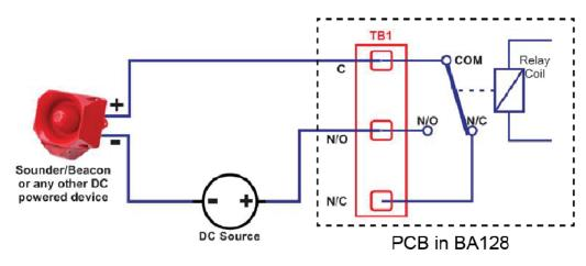
Figure 3 Control of DC Powered Ancillary Devices
