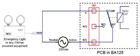
Figure 2 Control of AC Powered Ancillary Devices
