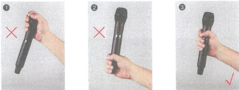
**Note 1:** Do not hold the transmitter grille with your hand, it's easy to block microphone to pick up the sound and cause changes.
