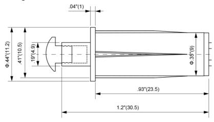
NOTE: Maximum plunger movement cannot exceed 0.23" (6mm) depth
