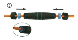
Lock the two waterproof plugs on the cable, then put them into the end of the long tube. Note: The plug is engraved with the word "waterproof" on one side outward.
