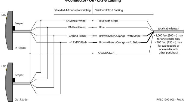
NXT-1R/-3R/-5R Exit Reader Installation Drawing 4-Conductor - OR - CAT-5 Cabling
