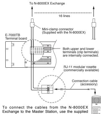
connection cable and a commercially available RJ-11 modular jack. These cables have no polarity.
