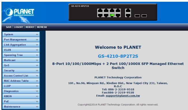
Figure 7-3: Web Main Screen of Managed Switch
