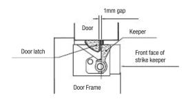
As drawn in the diagram above there should be a 1mm gap between the door latch and the front-face of the strike keeper, preventing the door from creating back pressure on the strike keeper when the door is closed.
