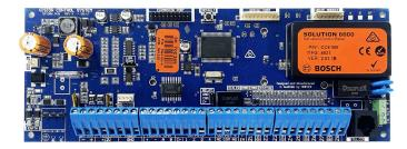
The Solution 6000 Access and intrusion alarm panel offers an extensive feature list including integrated proximity, numerous wire free options, high speed windows programming software and the simplest user / installer interface on the market today.
