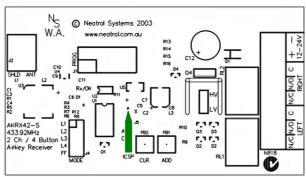
The remote learning socket must be removed before connecting an Airkey Programmer, Airkey Manager or using the manual ADD or CLEAR buttons.
