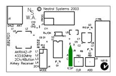
The remote learning socket must be removed before connecting an Airkey Programmer, Airkey Manager or using the manual ADD or CLEAR buttons.
