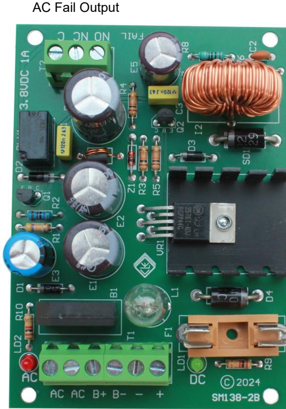
AC Input, Battery, DC Output
