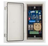
PCR43302240RE 2-Channel Receiver enclosed in an IP66 case
