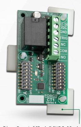
Trigger Current: -0.03 mA. @ 0V D.C., 0.9 mA. @ 12V D.C., 2.1 mA. @ 24V D.C., Operating Current: 8 mA. @ 12V D.C. (45 mA. with relay on), 10 mA. @ 24V D.C. (55 mA. with relay on), Operating Voltage: 10.5 - 28V D.C., Heavy duty 5 Amp. change over relay, 38mm x 72mm x 19.5mm (without feet), 50mm x 84mm x 23.5mm (with feet)
