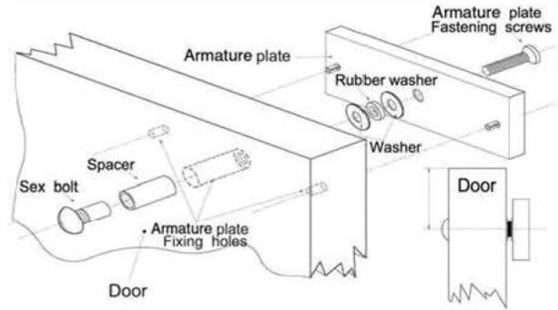
Armature plates must be installed with the components shown above. These components are provided with each electromagnetic lock.
