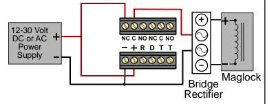
Another option is to install a diode, such as 1N4007, on the inductive load as shown in *Section 4.3.1 Basic Hookup*. Relay contacts shown with Switch 3 ON (Failsafe Mode) and Power On.
