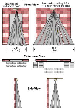
The higher the unit is mounted, the larger the coverage area. Do not mount the DS160/161 more than 15 ft. (4.6 m) above the floor.
