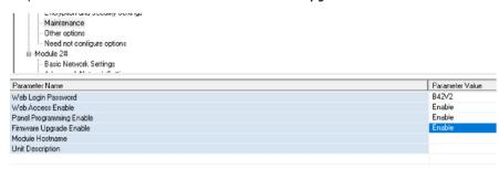
The panel MUST have *Firmware Upgrade Enable* set to **ENABLE** in AlinkPlus.
