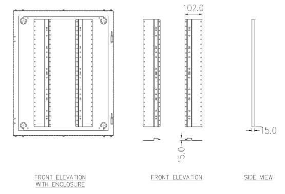
\*\*A- Actual length of the mounting rail, give in the table above. The mounting rail can be directly attached to the mounting rail studs installed in the enclosure.
