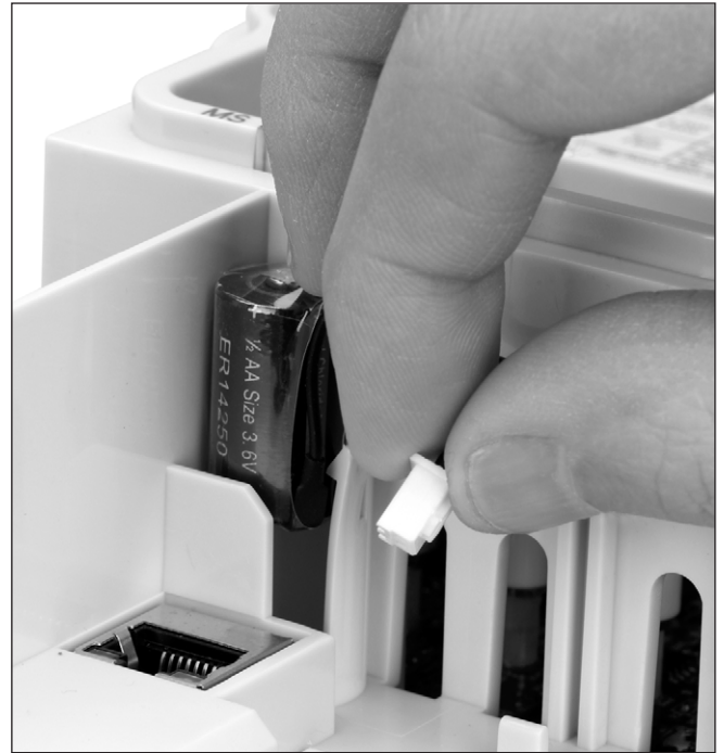
Figure 1. RTC battery connection
