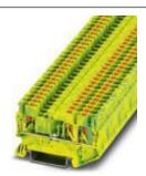
Ground modular terminal block, connection method: Push-in connection, number of connections: 3, cross section: 0.14 mm² - 4 mm², AWG: 26 - 12, width: 5.2 mm, height: 35.2 mm, color: green-yellow, mounting type: NS 35/7,5, NS 35/15
