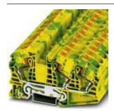
Ground modular terminal block, connection method: Push-in connection, number of connections: 3, cross section:  $0.5 \text{ mm}^2 - 25 \text{ mm}^2$ , AWG: 20 - 4, width: 12.2 mm, height: 53.3 mm, color: green-yellow, mounting type: NS 35/7.5, NS 35/15
