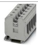
Feed-through terminal block, nom. voltage: 1000 V, nominal current: 125 A, connection method: Screw connection, number of connections: 2, cross section: 1.5 mm² - 50 mm², AWG: 16 - 1/0, width: 16 mm, height: 65.1 mm, color: gray, mounting type: NS 35/7,5, NS 35/15
